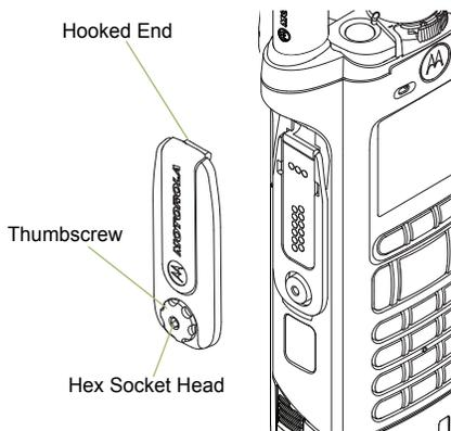
*To remove the accessory connector cover, rotate the thumbscrew counterclockwise until it disengages from the radio. If the thumbscrew is too tight, use an Allen wrench to loosen it first.*
