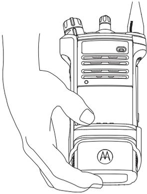
To remove the radio from the carry holder, place the tip of your fingers on the ledge of the carry holder and push at the bottom of the radio until the radio is released from it.
