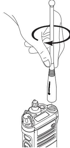
*To remove the antenna, turn the antenna counterclockwise. Make sure you turn off the radio first.*
