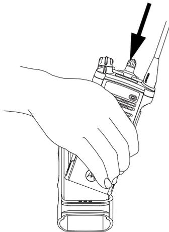
Position the radio within the carry holder with the main speaker facing outward. Slide the radio down into the carry holder until it clicks in place.
